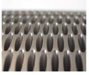
750 elliptical holes measuring 2.5 mm wide x 7 mm long x 4 mm deep are produced in a single 2-minute operation.
