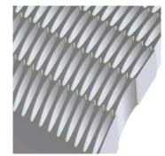
ECM permits holes to be machined into curved surfaces at oblique angles, which always leads to problems with conventional cutting methods.
